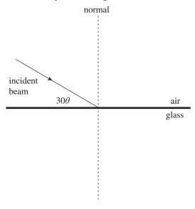
If the reflected beam and refracted beam are perpendicular to each other, what is the index of refraction of the glass?
