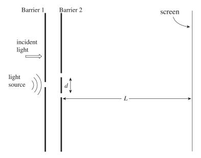
What is the purpose of the first (single-slit) barrier? Why not use two light sources, one at each slit at the second (a) barrier? Explain briefly.
